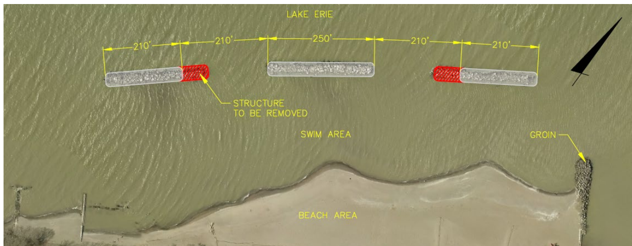
Figure 18: Breakwater Gap Widening Conceptual Plan
