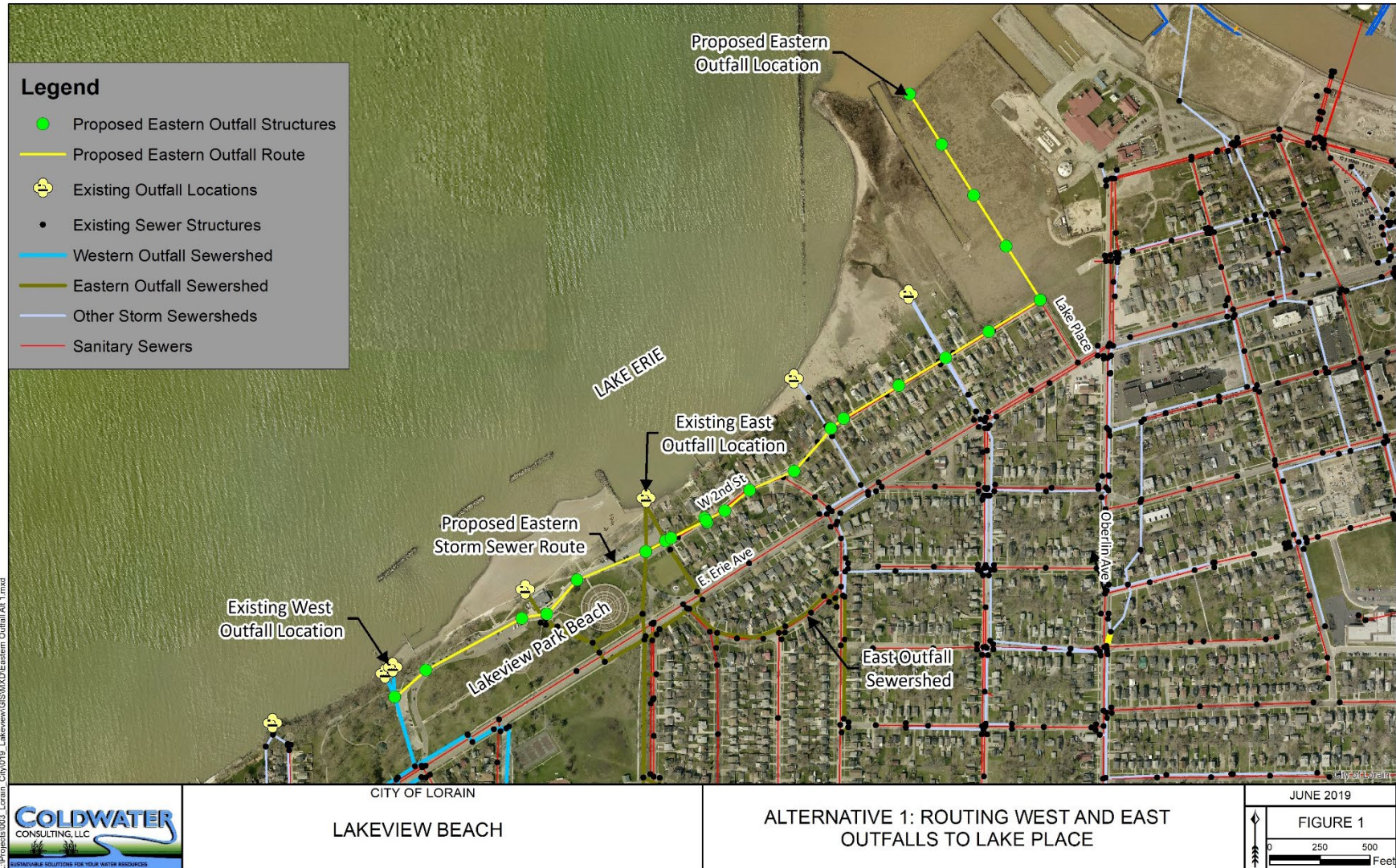
Figure 20: Alternative 1 - Routing East and West Outfalls to Lake Place
